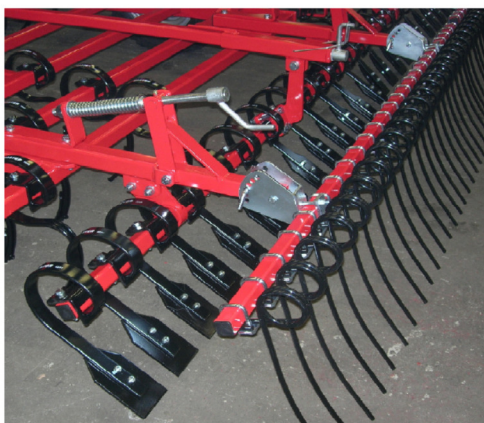
Control with a linkage bar
